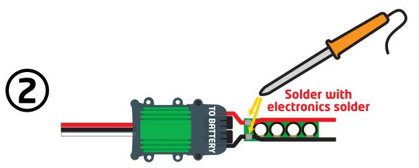
Solder the exposed power wires to the CC CapPack's posts using a high-power iron and electronics solder. Ensure that the RED wire is soldered to the (+) side and the BLACK wire is soldered to the (-) side.
