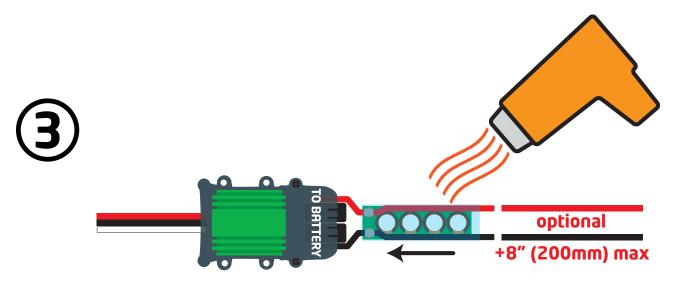
Slide the heat shrink over the CC CapPack and use a heat gun to shrink it. Up to 8 inches of additional wire may be added to the ESC wires.
