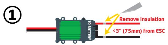
Remove 0.25 inches of insulation from the ESC's power wires within 3 inches of the ESC.
